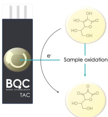
Similar to ET spectrophotometric TAC assays the BRS measurement is based on an electron transfer process from the antioxidants to the electrode.
