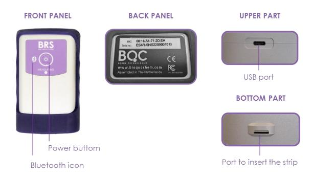
Power button. BRS Device is switched on and off by pressing the Power button. The ring around the Power button illuminates when the device is on. If the ring light is blinking the battery of the device is low.
